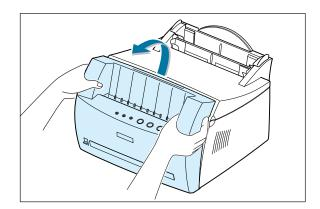
2 Remove the toner cartridge from its bag and remove the paper covering the toner cartridge completely out of the cartridge. Discard the paper.
